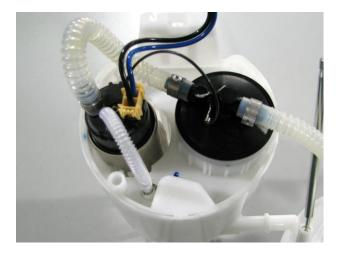
8 – reinstall the assembly top-hat to the center/buckets assemblies and connect the electrical connector harness to the hat assembly. Reinstall the fuel level sender and connector the electrical connector to the assembly top-hat
